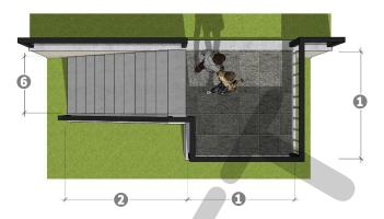
①: MINIMUM OF EIGHT (8) FOOT BY EIGHT (8) FOOT LANDING; ②: VARIABLE LENGTH STAIRCASE; ③: WROUGHT IRON OR BLACK TUBLAR STEEL; ④: NATURAL STONE, BRICK, OR CONCRETE MATCHING THE RETAINING WALL; ⑤: VARIABLE HEIGHT BUT A MINIMUM OF THREE (3) FEET; ⑥: MAXIMUM OF SIX (6) FEET.
