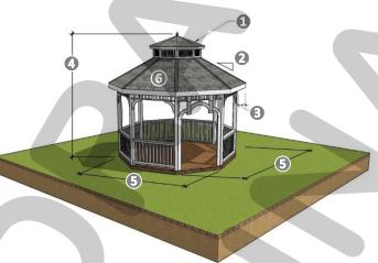
①: CUPOLA OR CLERESTORY; ②: 2:1 MINIMUM ROOF PITCH; ③: 1.5-FOOT MAXIMUM OVERHANG; ②: 18-FEET MAXIMUM HEIGHT WITH A CUPOLA OR CLERESTORY AND 15-FEET WITHOUT A CUPOLA OR CLERESTORY; ⑤: 12-FEET MAXIMUM; ⑥: ROOF CAN MATCH THE PRIMARY STRUCTURE OTHERWISE THE ROOF SHALL BE STANDING SEAM METAL.
