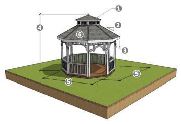
①: CUPOLA OR CLERESTORY; ②: 2:1 MINIMUM ROOF PITCH; ③: 1.5-FOOT MAXIMUM OVERHANG; ②: 18-FEET MAXIMUM HEIGHT WITH A CUPOLA OR CLERESTORY AND 15-FEET WITHOUT A CUPOLA OR CLERESTORY; ⑤: 12-FEET MAXIMUM; ⑥: ROOF CAN MATCH THE PRIMARY STRUCTURE OTHERWISE THE ROOF SHALL BE STANDING SEAM METAL.
