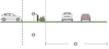
●: MINIMUM THREE (3) FOOT MASONRY WALL; ②: 20-FOOT LANDCSAPE BUFFER; ③: STREET OR ALLEYWAY
