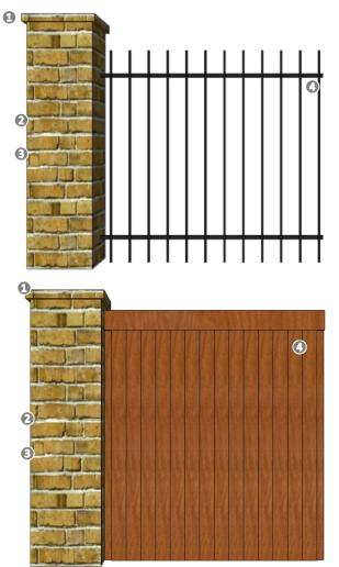
Rowlock Cap; 2: Running Bond; 3/8" Tooled Joints (*Typical*);
