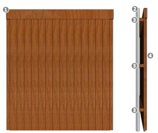
1 Top Rail; 2: Galvanized or Stainless-Steel Post (*Recommended Minimum of* 2.375");
