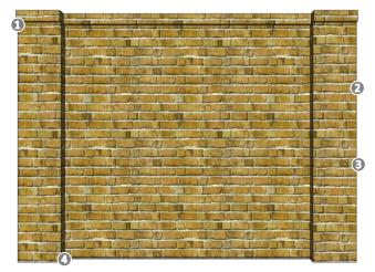
Rowlock Cap; 2: Running Bond; 3: 3/8" Tooled Joints (*Typical*);
