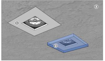
●: FLUSH LENS (*I.E. FULLY RECESSED*); ②: PROJECTING LENDS (*I.E. NOT FULLY RECESSED*); ③: CEILING
