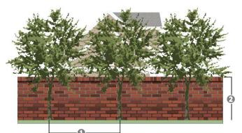
●: CANOPY TREES 20-FOOT ON CENTER; ②: MINIMUM SIX (6) FOOT MASONRY WALL:
