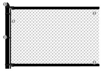
Post Cap; 2: Top Rail; 3: Bottom Rail; 4: Tension Band;
