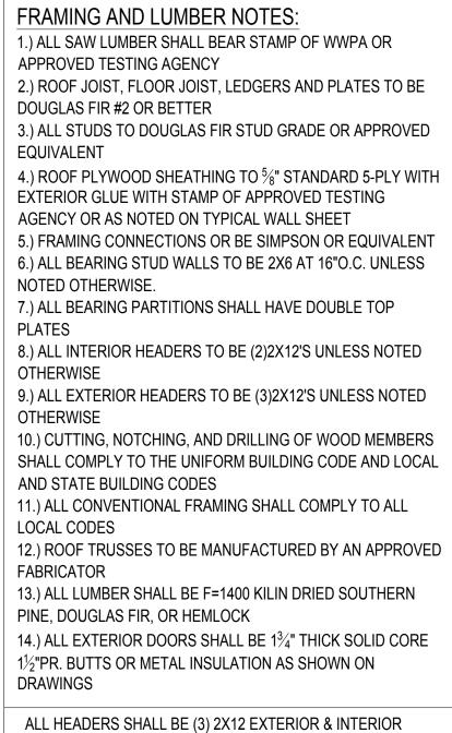
BEARING WALLS UNLESS NOTED OTHERWISE. MIN.-1-JACK STUD EA. SIDE OF OPG. TO 6' WIDE MIN.-2-JACK STUD EA. SIDE OF OPG. TO 8' WIDE MIN.-3 JACK STUD EA. SIDE OF OPG. TO 12' WIDE ALL HEADERS (ANY SIZE) SHALL BE <sup>1</sup>/<sub>2</sub>" PLYWOOD FILLERS. GLUE & NAILED W/ 16D NAILS
