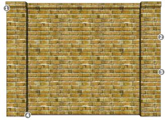
1: Rowlock Cap; 2: Running Bond; 3: 3/8" Tooled Joints (*Typical*); 2: Concrete Footing/Mow Strip.
