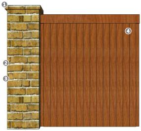
1: Rowlock Cap; 2: Running Bond; 3: 3/8" Tooled Joints (*Typical*); 3: Wrought Iron or *Board-On-Board* Wood Fence.
