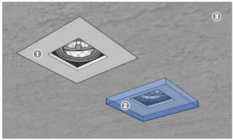
①: FLUSH LENS (I.E. FULLY RECESSED); ②: PROJECTING LENDS (I.E. NOT FULLY RECESSED); ③: CEILING
