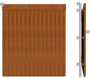
①: Top Rail; ②: Galvanized or Stainless-Steel Post (*Recommended Minimum of* 2.375"); ③: Stinger Board (Recommended Minimum of 2" x 3"); ④: Minimum ½" Wood Screen.
