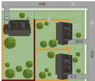
1: PORCH; 2: 20-FOOT BUILD LINE; 3: TEN (10) FOOT BUILD LINE; 2: STREET; 3: ALLEYWAY; REAR YARD FENCE; SIDE YARD FENCE
