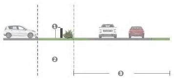
●: MINIMUM THREE (3) FOOT MASONRY WALL; ②: 20-FOOT LANDCSAPE BUFFER; ⑤: STREET OR ALLEYWAY
