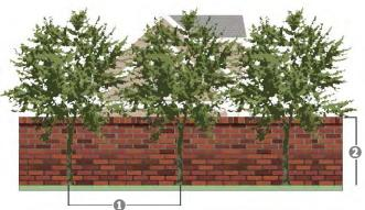
①: CANOPY TREES 20-FOOT ON CENTER; ②: MINIMUM SIX (6) FOOT MASONRY WALL:
