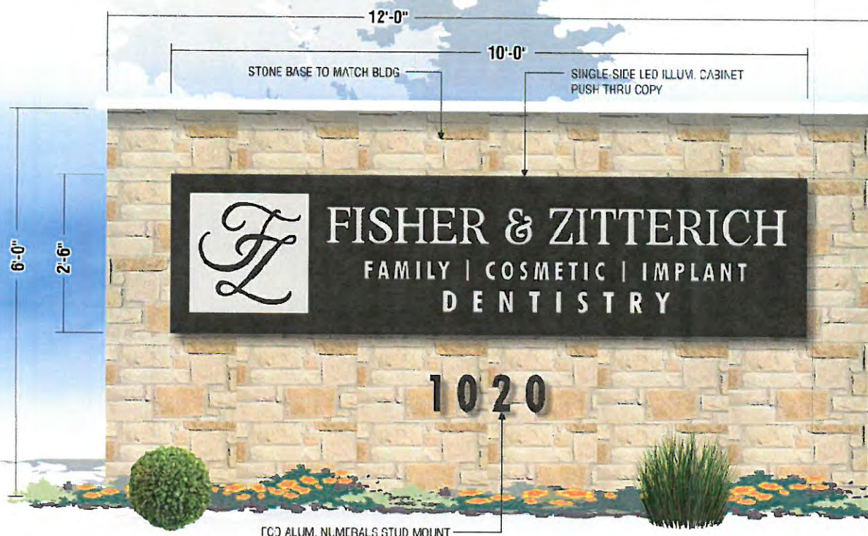
SIGN C FACE VIEW: V-SHAPED INT. ILLUM. MONUMENT SIGN SCALE: 3/4" = 1'-0"
