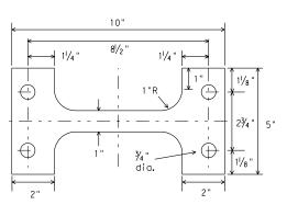
BOLT KEEPER PLATE 30 Ga galv. sheet steel
